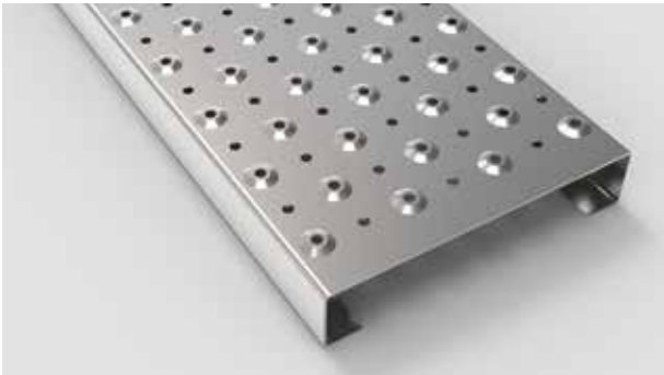
Type AP 2 - 50 with drainage (MAA) Type AP 3 - 50 with drainage (MAA) Embossed dome with Ø 8 mm perforation punched up 3 mm high. Drainage perforation flat Ø 8 mm both on a 50 mm c.t.c staggered pitch.
