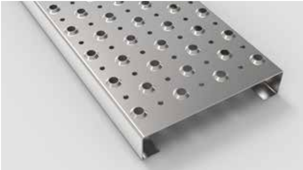
Type AP 2 - 50 with drainage (MAW) Type AP 3 - 50 with drainage (MAW) Anti-slip perforation Ø 14 mm punched up 4 mm high. Drainage perforation flat Ø 8 mm both on a 50 mm c.t.c staggered pitch.
