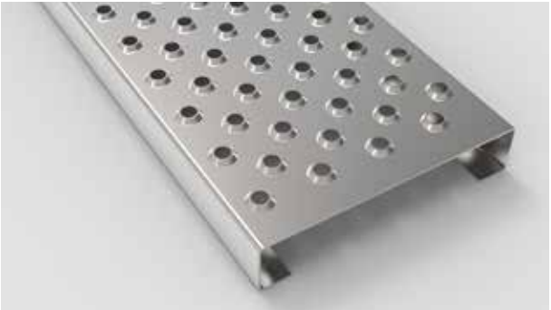
Type AP 2 - 40 without drainage (ZAW) Type AP 3 - 40 without drainage (ZAW) Anti-slip perforation Ø 14 mm punched up 4 mm high on a 40 mm c.t.c staggered pitch. No drainage holes.
