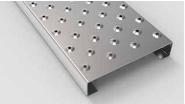
Type AP 2 - 50 without drainage (ZAA) Type AP 3 - 50 without drainage (ZAA) Embossed dome with Ø 8 mm perforation punched up 3 mm high. No drainage holes.
