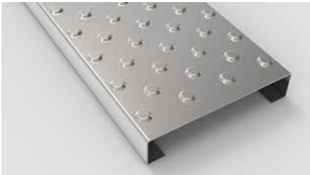
Type AP 2 - 50 closed (NOP) Type AP 3 - 50 closed (NOP) Embossed Ø 16 mm dome 4 mm high on a 50 mm staggered pattern. Also available with drainage perforation Ø 8 mm if required.
