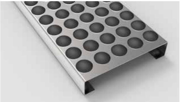
Type AP 2 - 50 rubber caps (DOP) Type AP 3 - 50 rubber caps (DOP) Perforation Ø 14 mm, c.t.c. 50 mm, 4 mm deep, also with drainage perforation Ø 8 mm if required, c.t.c. 50 mm, 0 mm deep. Suitable for using rubber caps. Preferred widths in multiples of 50 mm.
