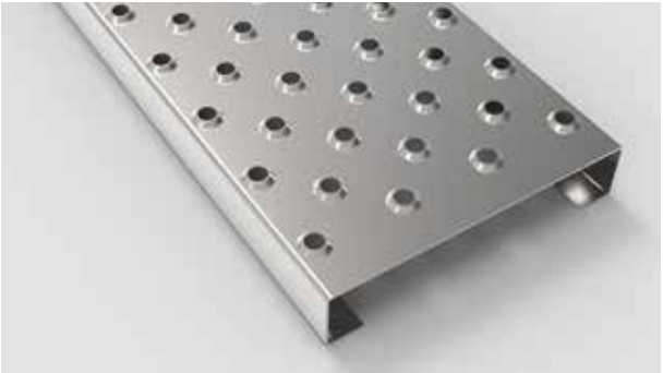
Type AP 2 - 50 without drainage (ZAW) Type AP 3 - 50 without drainage (ZAW) Anti-slip perforation Ø 14 mm punched up 4 mm high on a 50 mm c.t.c staggered pitch. No drainage holes.
