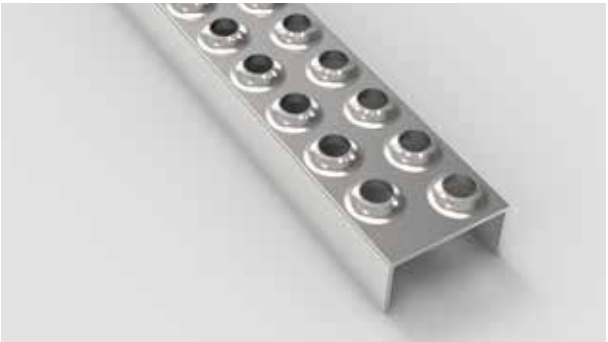
Type AP 2 - 50 ladder rung (LAD2) Anti-slip perforation Ø 12 mm, c.t.c. 25 mm, 5 mm high. Width 50 mm, height setting 37 mm.
