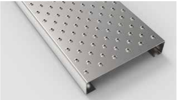
Type AP 2 - 30 safety without drainage (VZA) Anti-slip perforation Ø 5 mm punched up 3 mm high on a 30mm c.t.c staggered pitch. No drainage perforations.
