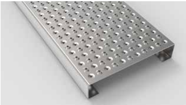
Type AP 2 - 30 safety with drainage (VMA) Anti-slip perforation Ø 5 mm punched up 3 mm high. Drainage perforation Ø 5 mm punched down 3 mm deep both on a 30 mm c.t.c staggered pitch.
