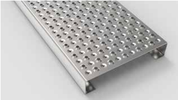
Type AP 2 - 30 with drainage (MAW) Anti-slip perforation Ø 8 mm punched up 3 mm high. Drainage perforation Ø 5 mm punched down 3 mm deep both on a 30 mm c.t.c staggered pitch.
