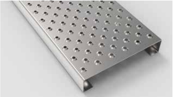
Type AP 2 - 30 without drainage (ZAW) Anti-slip perforation Ø 8 mm punched up 3 mm high on a 30mm c.t.c staggered pitch. No drainage perforations.
