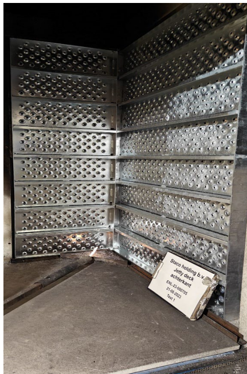
Photographs 1 and 2: Specimen Deck series test 1 prior to testing
